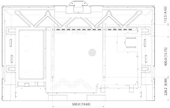
Figure 3-8 Attach the vertical brackets (65-inch series) (mm [inch])
