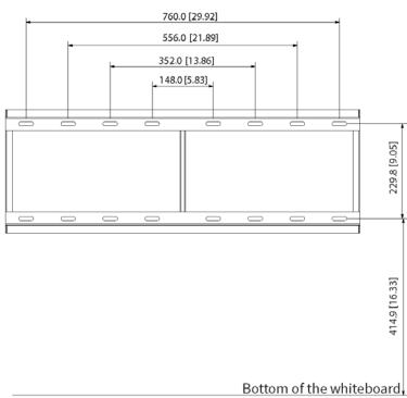
Figure 3-5 Installation dimensions (98-inch series) (mm [inch])
